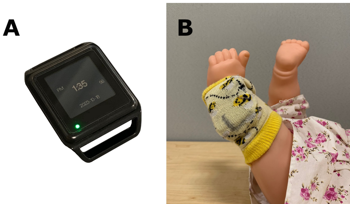
Fig 1. Opal sensors worn on an infant. (A) A wearable sensor used in each recording. (B) Custom-made legwarmers with sensors inserted put on each ankle of an infant.
